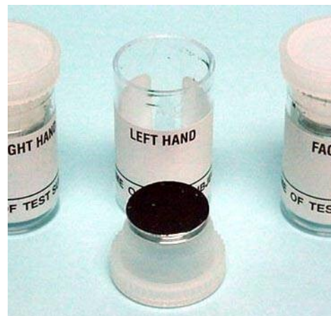
The collection device of a GSR kit for the left hand.
