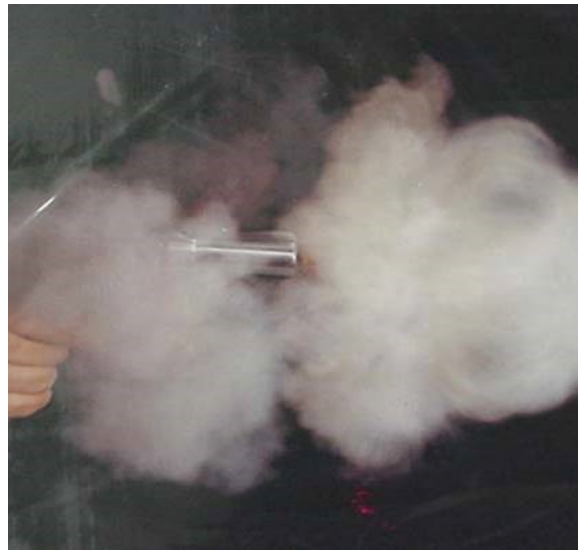
An example of the residues expelled from a firearm during the firing process.
